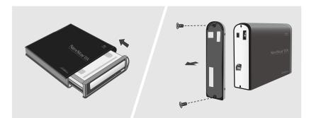
7. Slide the tray back into enclosure and install the back panel
