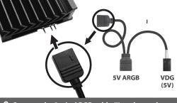
9. Connect the 3-pin ARGB cable (I) to the card.
