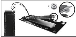
4. Align your M.2 Module with the M-Key interface to the RBG card M.2 connector, insert your NVMe module into the connector, put on the M.2 holding Nut (J) on your NVMe as shown.
