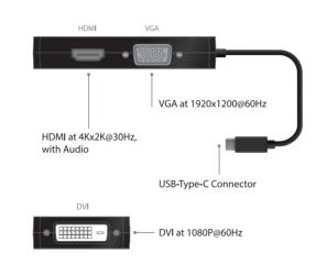
Connect device (Support only one video interface at a time)
