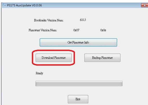
**Step5:** Browse to where “ps176b0\_0x07.0x00.0x26\_encrypt\_bank12.hex” file is located and select open to select the firmware file.
