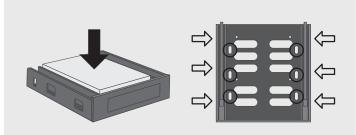
**5b.** To install 3.5" hard drive, place 3.5" drive as shown and secure either from the bottom or from the side using hole align with the drive mount.
