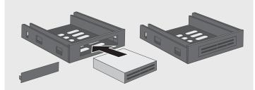
5a. To install 3.5" Card reader or other device, remove front plate cover and insert device into the 3.5" drive bay. Align the device front and secure using instruction from the device installation guide.
