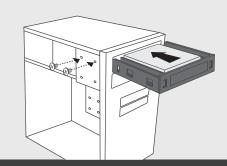
6. Slide the mounting bracket into the system chassis until the front panel is flush with the front of the case. Secure the 5.25" device using the provided screws on both side.
