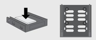
4. Mount the 2.5" SSD or HDD into the bay shown and secure from the bottom using the provided screws on the mounting hole shown.
