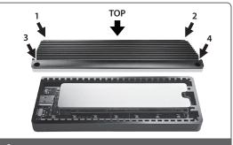
Place back the casing and RGB LED Layer remove in step #1, and secure using the 4 screws you removed in Step #1.
