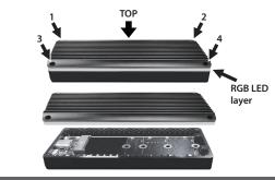
Note the TOP casing cover is closes to the RGB LED Layer. Remove the 4 screws shown using the screwdriver and lift off the TOP casing cover and RGB LED layer.
