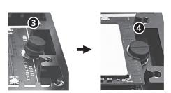
3. ① Insert your M.2 NVMe into the M.2 socket, your M.2 is keyed with a notch that aligns with the socket. Insert into the socket at an angle, ② push down the M.2 NVMe.
