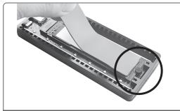
Remove the film protecting the Thermal pad on both sides and place the Thermal pad on top of your M.2 NVMe as shown.
