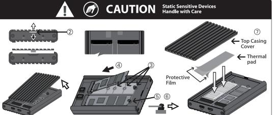
2) This is a toolless unit, use your finger to pry it apart via the slot shown to lift off the top cover.
