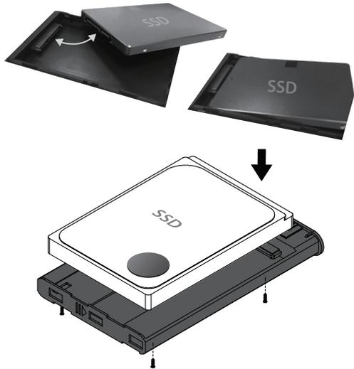
4) Mount your SSD/HDD. Align your SSD/HDD SATA interface with the SATA interface on the tray, and insert at a slight angle for the Drive SATA interface to mate with the SATA interface on the Tray. Insert the drive until the SATA interface is fully connected. Once the SATA interface is fully mated, the drive will sit flat into the tray. Secure using the provided 4 screws from the underside.
