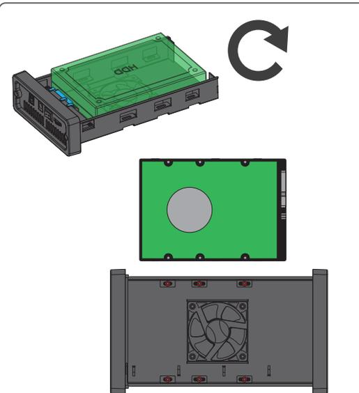
6. While holding the drive to the Tray, flip over to the underside of the tray and secure using the provided screws to 4 of the aligned holes.
