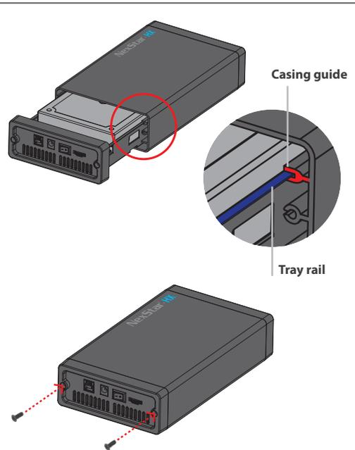
7. Align the tray with the mounted drive to the casing guide to the tray rail and slide back the Tray and secure using the 2 screws.
