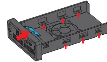
4. Note the Parts layout, location of the SATA connector on the inside of the Tray and the hard drive mounting hole.
