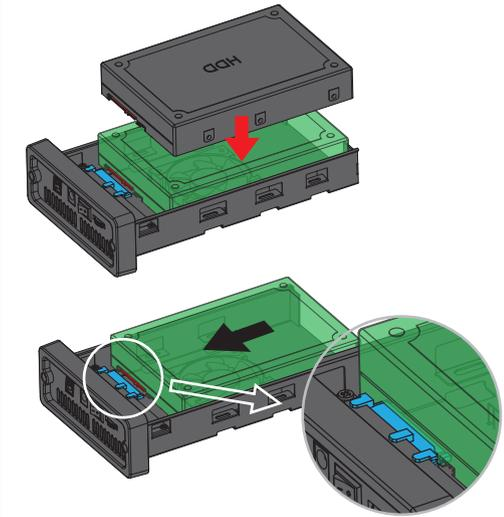
5. Place your 3.5" Hard drive horizontally down shown by the arrow. Note the orientation of the SATA connector on the drive. Once place down push the drive in the direction of the arrow for the SATA connector on the Tray to mate with the SATA connector on the drive. Make sure it is making good contact for the SATA drive to function correctly.
