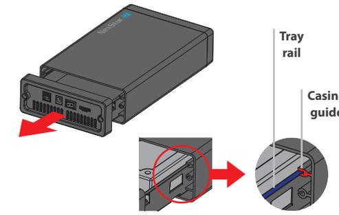
3. Slide out the tray from the enclosure casing. Note the guide on the casing where the tray rail slide out.
