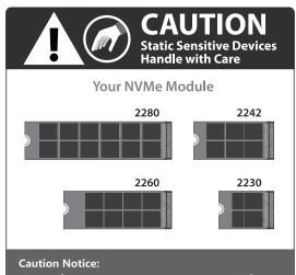
This enclosure supports an M.2 NVMe module only; it is NOT designed for other NON-NVMe M.2. Your M.2 Module may come in different sizes like
