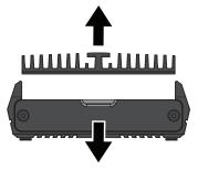
2 This is a tooless enclosure, note the arrow shown to separate the top cover Plate.
