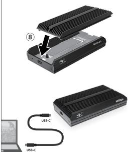
8 Slide the top cover at an angle and close the top cover. The Storage is ready.
