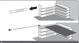
7. Locate a free PCIe x4, x8 or x16 expansion slot and remove the plate covering the back aligned with the PCIe slot. Insert this new PCIe card into the PCIe slot, make sure the PCIe card contacts is totally inserted into the PCIe slot. Secure and fasten the PCIe card as documented in the Computer System manufacturer's documentation.
