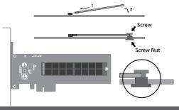
4. Attached the M.2 module by inserting the M.2 Card at an angle, push it down and secure with the Screw Nut from the bottom and the screw from the top down to hold the M.2 module in place.
