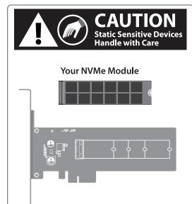
Before you unpack your NVMe module and take out the PCle card, please be aware that these are sensitive devices and can be damaged by Static Electricity.
