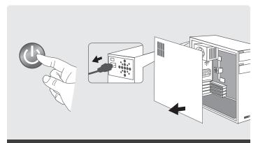
2. Turn off Computer System, unplug power and remove the cover of the **Computer System**
