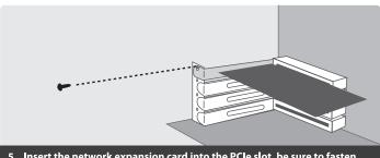
5. Insert the network expansion card into the PCIe slot, be sure to fasten the bracket as documented in the computer case manufacturer's documentation.
