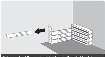
3. Locate a free PCIe expansion slot and remove the metal L bracket
