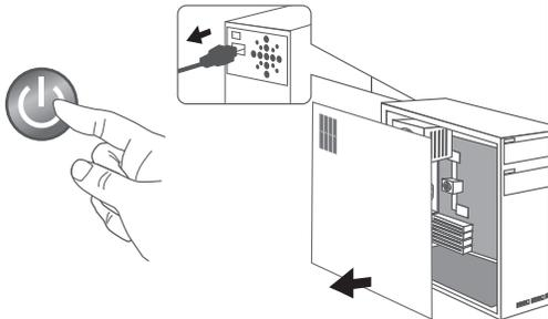
5. Turn off the Computer System, MUST unplug the computer power cord from the wall outlet, wait 1-2 minutes, and remove the cover of the Computer System.
