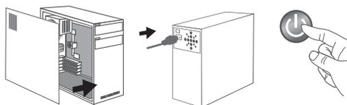
7. Place the case cover back on the Computer System. Reattached the power cord to the Computer System, plug back to the wall outlet, and power ON the System.
