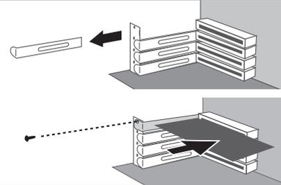
6. Locate a free PCIe X4, x8, or x16 expansion slot and remove the plate covering the back aligned with the PCIe slot. Insert this new PCIe card into the PCIe slot, make sure the PCIe card contacts are fully inserted into the PCIe slot. Secure and fasten the PCIe card as documented in the Computer System manufacturer's documentation.
