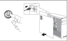
Turn off the Computer System, MUST unplug the computer power cord from the wall outlet, wait 1-2 minutes, and remove the cover of the Computer System.
