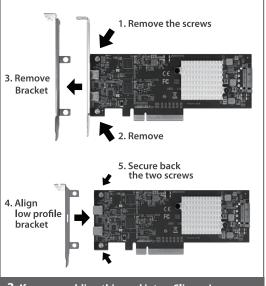
3. If you are adding this card into a Slim or Low Profile System, please replace the standard bracket with a Low Profile Bracket provided. Remove the two screws holding the standard bracket, replace it with the Low Profile Bracket and secure back the two screws holding the bracket.
