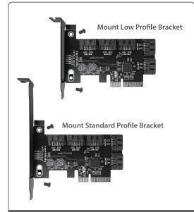
4. If your system is a slim or low profile system, please use the provided Low Profile bracket. If your system is a standard desktop or tower chassis, please use the provided Standard Profile bracket. Secure the right bracket using the screws provided to the card.
