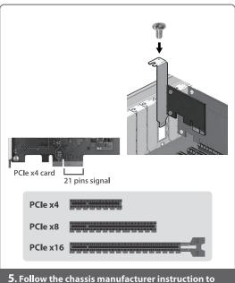
5. Follow the chassis manufacturer instruction to select and align this card with the right PCle slot. Insert the card secure the card to the chassis. This is card requires a PCle x4 slot to function correctly, it must be inserted into a working x4 slot or better like x4 or x8 or x16 slot.
