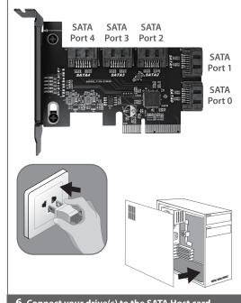
Connect your drive(s) to the SATA Host card. Replace chassis side panel or cover, connect power back to the wall outlet.
