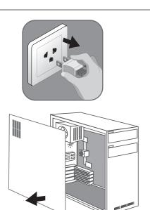
Make sure your system power is OFF, unplug the system power from the wall outlet, and wait a whole minute. Remove the side panel or cover for your system by following the instruction from the chassis manufacturer.
