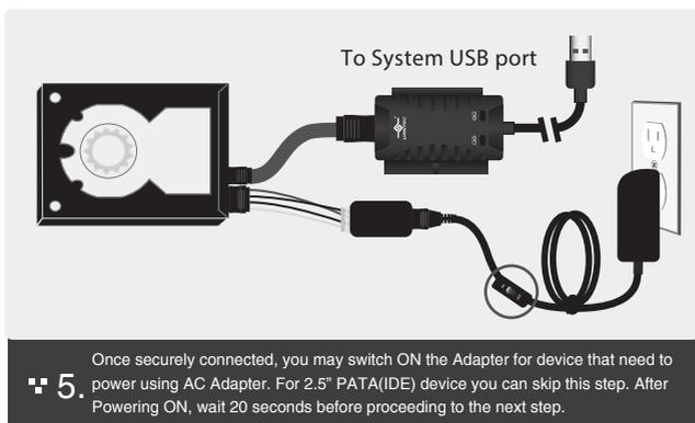
❖ 5. Once securely connected, you may switch ON the Adapter for device that need to power using AC Adapter. For 2.5" PATA(IDE) device you can skip this step. After Powering ON, wait 20 seconds before proceeding to the next step.
