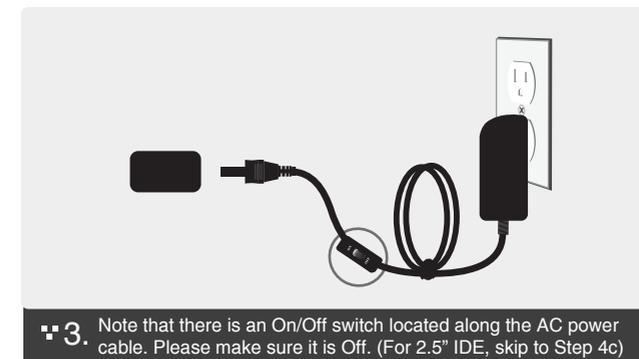
❖ 3. Note that there is an On/Off switch located along the AC power cable. Please make sure it is Off. (For 2.5" IDE, skip to Step 4c)
