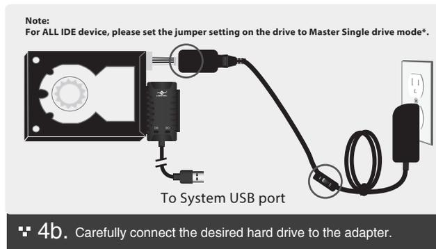
❖ 4b. Carefully connect the desired hard drive to the adapter.
