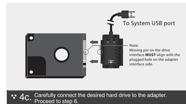
❖ 4c. Carefully connect the desired hard drive to the adapter. Proceed to step 6.
