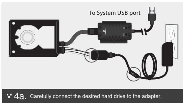
❖ 4a. Carefully connect the desired hard drive to the adapter.
