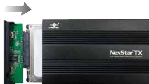
5-3 Secure the caddy to the housing using the screws provided.
